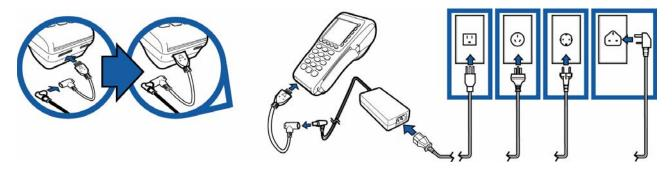
Figure 19 V<sup>x</sup>670 Power Pack Connection
